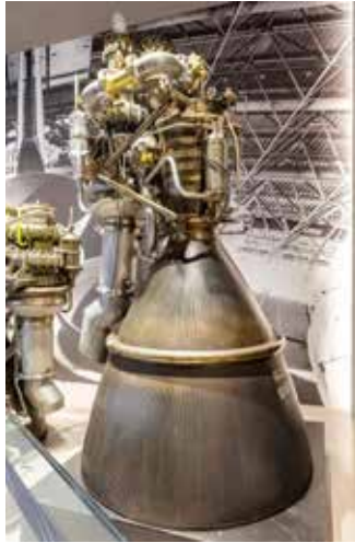
“长征”系列火箭二级发动机 Second-stage engine used in the Long March rocket series
