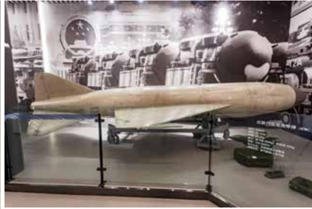
“上游一号”舰舰导弹 弹长：6.55m；弹径：0.76m；翼展：2.41m；弹重：2095kg SY-1 Ship-to-Ship Missile Length: 6.55m; Diameter: 0.76m; Wingspan: 2.41m; Weight: 2,095kg
